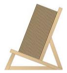
Stacking on edge should be avoided whenever possible. Where space will only permit edge stacking then the edges should not be permitted to come into direct contact with the floor to avoid possible moisture pick-up or damage to the edges.
